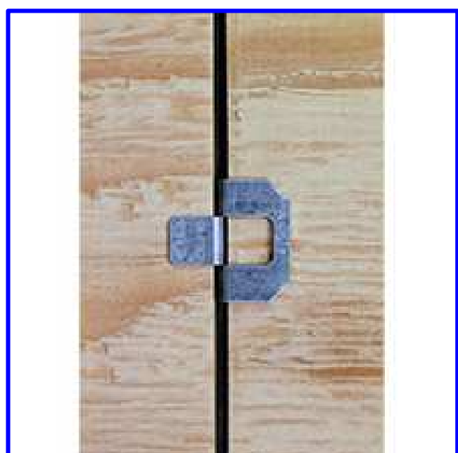
PANEL SHEATHING CLIPS PSCL 1/2 USE WITH PLYWOOD 24" OC NOT NEEDED @ 16" OC UNLESS SHEETING IS LESS THAN 24" IN WIDTH THEN ONE CLIP IS REQUIRED IN EACH BAY
